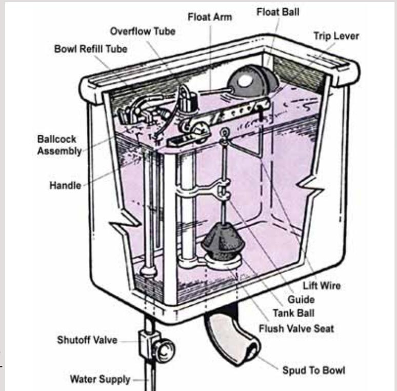
**Step 1:** Lift up on the float arm. If the water stops, you know the problem is that the float ball doesn't rise far enough to lower the valve plunger in the ballcock assembly. One reason could be that the float ball is rubbing against the side of the tank. If this is the case, bend the float arm slightly to move the ball away from the tank side.
